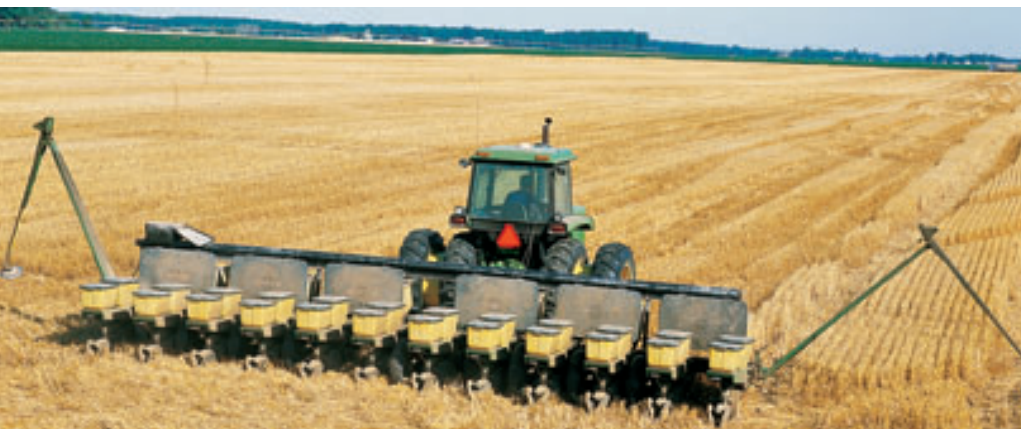
Figure 11 ► This farmer is practicing no-till farming. The tractor plants a new crop by poking seeds into the soil through the remains of the old crop.
