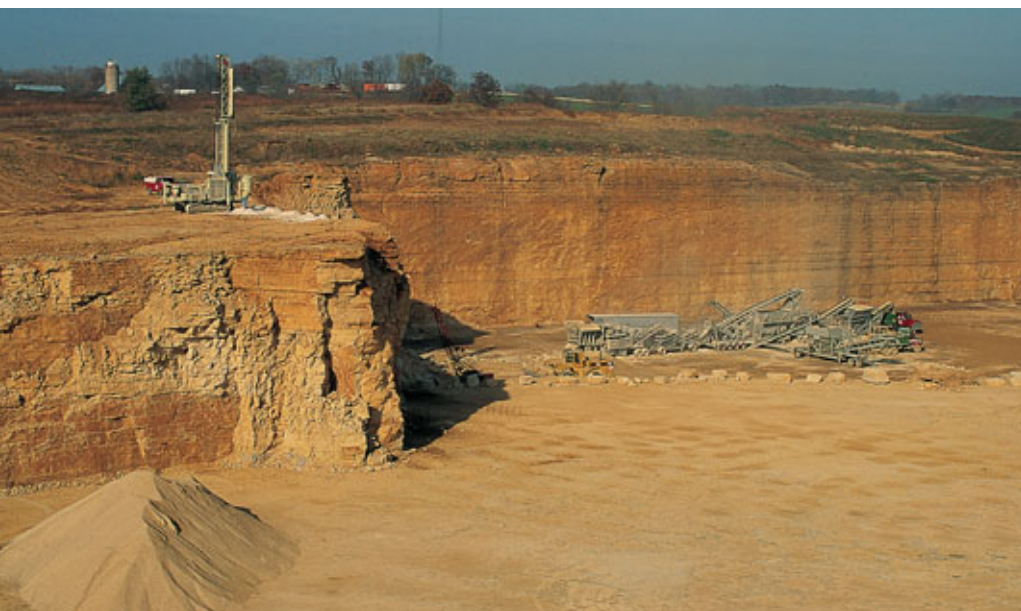
Figure 10 ► Open pits called quarries are used to mine near-surface materials such as building stone, crushed rock, sand, and gravel.
