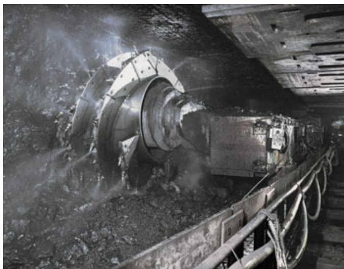
Figure 8 ► Heavy equipment, like the rotating shearer of the longwall mining system shown here, is used to remove coal in subsurface mines.
