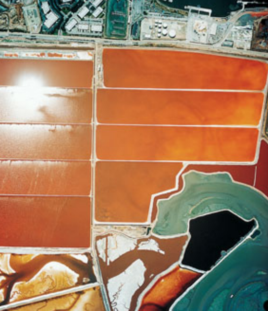
Figure 11 ► This is an aerial view of solar evaporation ponds that are used to produce salt on San Francisco Bay.
