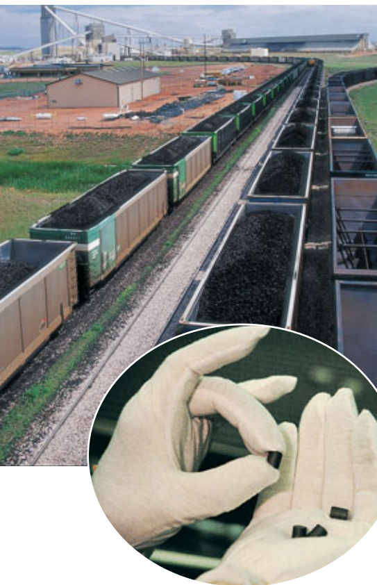
Figure 16 ► Uranium is a very compact fuel. The uranium pellets (above) can generate as much electricity as the trainload full of coal does.
